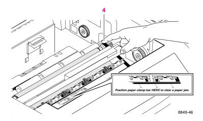
**Caution** Do not force or pull the jammed paper out of the paper clamps. This will damage the printer. You must first release each paper clamp and gently remove the paper.
