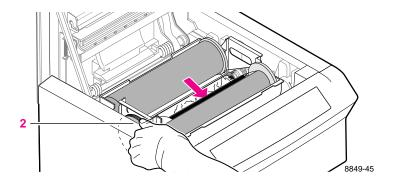
Lift out the transfer roll tray. Check the roll for tears and wrinkles. (If the roll is damaged, replace it with a new one.) Straighten the roll and make sure that the axles on the endcaps are set snugly into the tray. 4. To check the paper clamp bar, pull on the black rubber belt until the paper clamp bar is positioned over the label Position paper clamp bar HERE to clear a paper jam. If the paper clamps are holding any paper, this is the cause of the jam.
